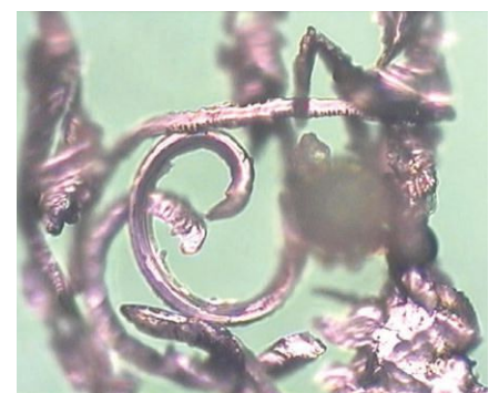
Figure 4 | Ferrogram: three-body abrasive wear due to foreign particles in the oil.
