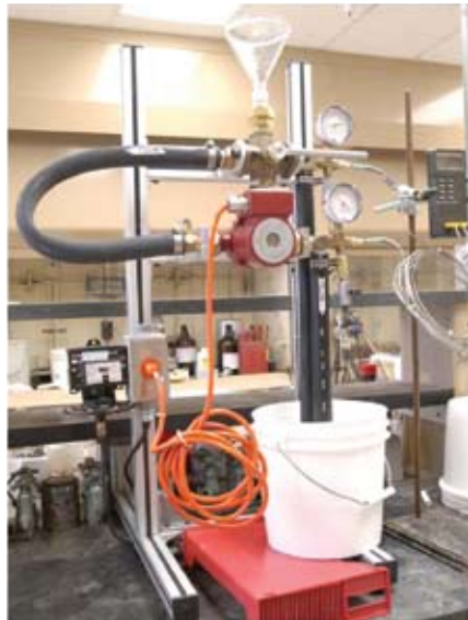
Industry Standard ASTM D3035 1" ID HDPE Pipe & brass stab fittings. Max temp 109 F.
