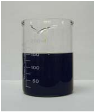
Figure 5 | Nanoparticles dispersed in heat transfer fluids have the potential to improve thermal conductivity. [Courtesy of Dynalene Inc.]
