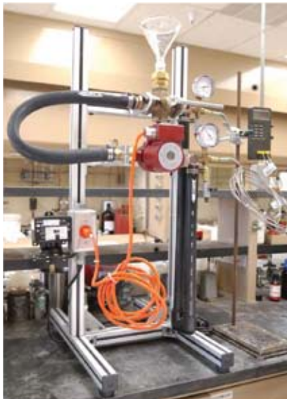
Grundos 85W Centrifugal Pump. Flow rate 4 gpm.
