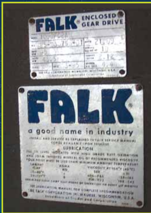
Figure 11. Gear drive faceplate label showing viscosity parameters
