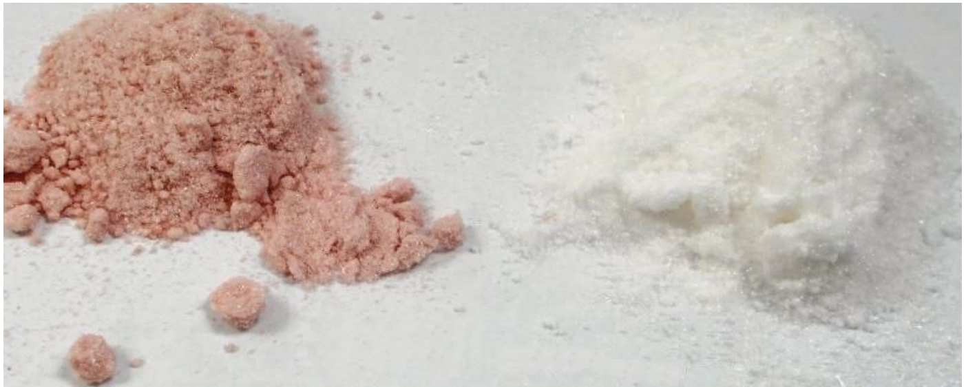
Figure 1 | HX-1 additives can exhibit different levels of purity. The image on the left represents an additive with a noticeable color and offensive odor. Purification produces an additive with higher purity, which is noted by the white. (Figure courtesy of Novitas Chem Solutions, LLC.)
