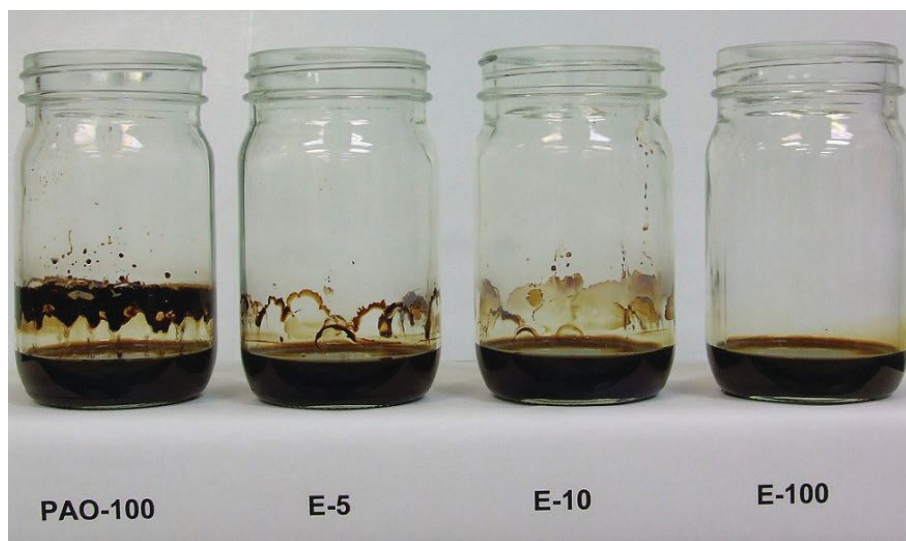
Figure 2 | Jars showing results from the thermal stability testing of PAO (PAO-100), a synthetic ester with the same viscosity (E-100) and blends of 5% (E-5) and 10% (E-10) of the ester in PAO at 260 C for 20 hours are shown. E-100 shows superior thermal stability as compared to PAO-100, but introduction of small percentages of ester (E-5 and E-10) to PAO leads to an improvement in thermal stability. (Figure courtesy of Zschimmer & Schwarz, Inc.)
